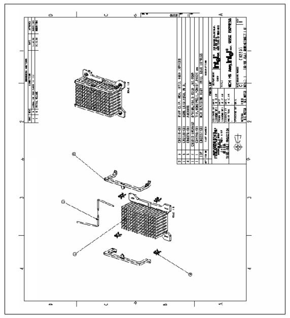
Figure 8-1. Plastic Wave Soldering Heatsink Assembly Drawing
